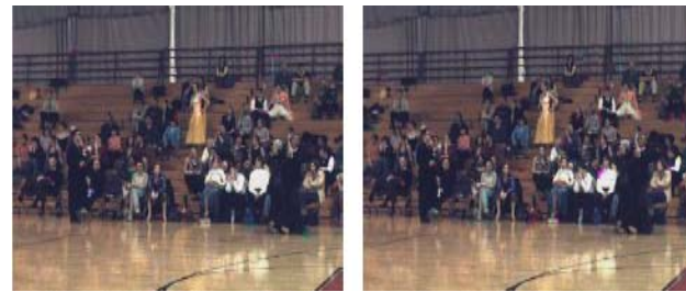
Fig. 5 TDEC (left) and STDEC (right) concealed I-frame No.241 of the test sequence “Ballroom” with packet loss rate (PLR) = 20%
