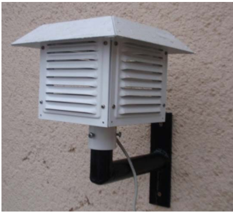
Fig. 2 Fog sensor – outdoor unit
