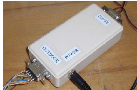
Fig. 5 Fog sensor – internal (indoor) unit
