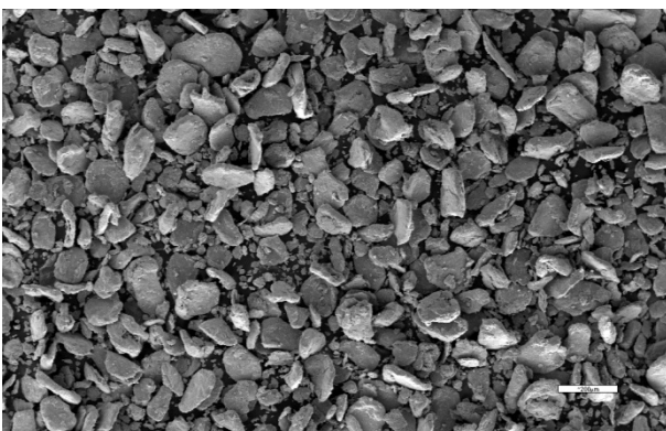
Fig. 2 Fracture of the milled Vitroperm sample L observed by SEM
