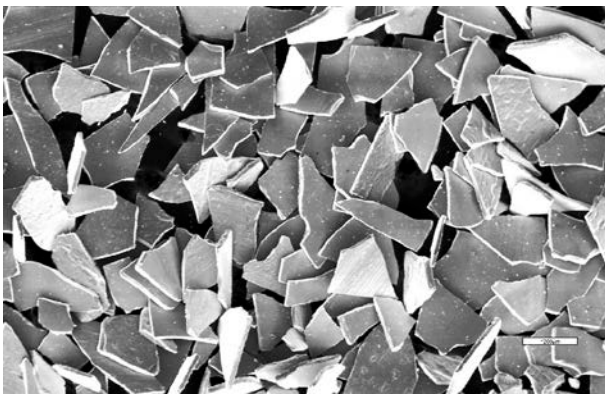
Fig. 6 Fracture of the sample Somaloy®700 powder observed by SEM
