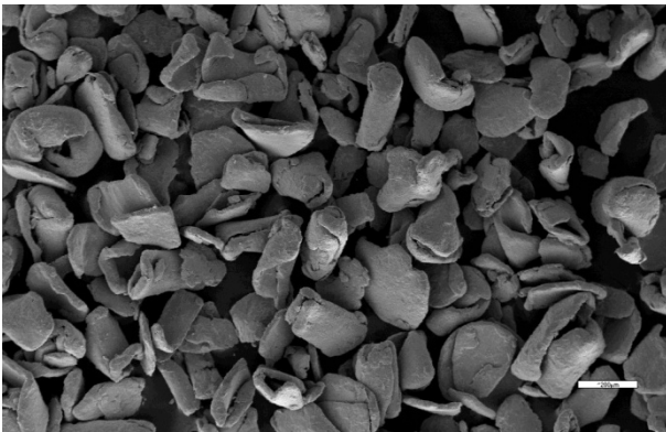
Fig. 1 Fracture of the milled Vitroperm sample R observed by SEM
