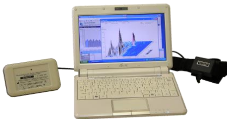
Fig. 3 Microcomputer system for non-invasive examination of the autonomic nervous system DiANS PF8
