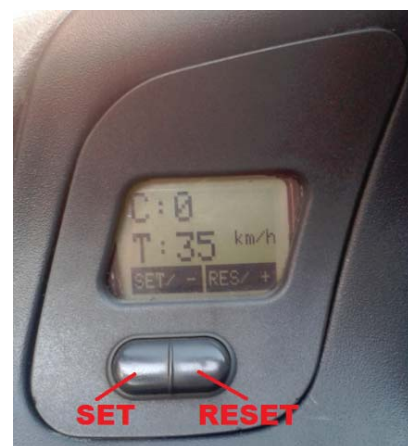
Fig. 4 "SET" and "RESET" buttons for control of the cruise control with current and target speed on a display
