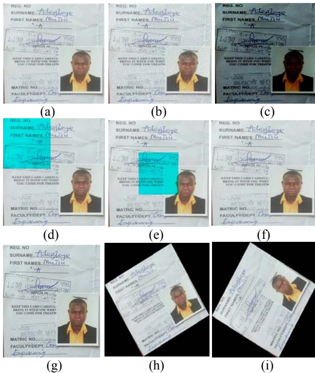
Fig. 6 Images with attacks for (a) Gaussian noise, (b) Pepper and salt noise (c), Sharp enhancing, (d) Image cutting (1/4 edge), (e) Image cutting (1/4 center), (f) Low-pass filter, (g) Image rotation (300) and (h) Image rotation (600)
